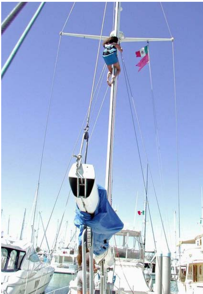
The bearing allows the mainsail to furl inside the mast.
