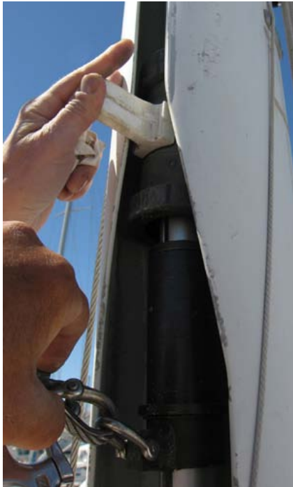
The bearing allows the mainsail to furl inside the mast.
